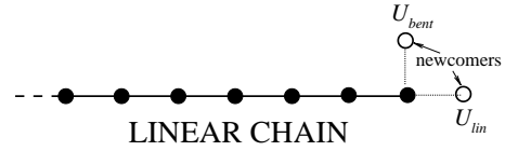
Fig. 6. The possible newcomers at the edge of linear chain with repulsive energies of U_{\text{lin}} (see Eq. (5)) for linear configuration of type (2) (Fig. 3) and U_{\text{bend}} (see Eq. (12)) for bent configuration of type (3) (Fig. 3).
